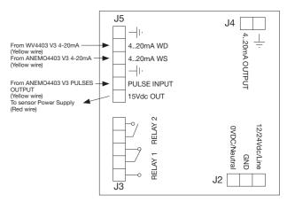
J3: Output relays connector. Configuration through PO9 y P16. J4: Analogue output connector. Configuration through P24 y P25.
