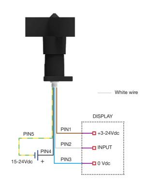
Colour wires referenced to the cable supplied.
